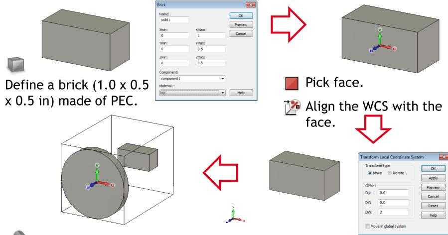
Define a cylinder (outer radius: 1.0 in, height: 0.25 in) made of PEC.
