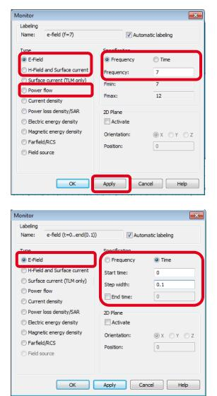
Define E-field, H-field and Power Flow monitors at 7 GHz and 12 GHz.
